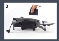
Insert the Automoving light Battery into the Automoving light's battery slots. Slide the battery forwards to the Automoving light's battery compartment.
