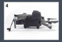
Make sure the battery is mounted securely and that the battery latches have clicked into place. The image illustrates a correctly mounted battery. There should be no «GAP» between the battery and the battery connector on the Automoving light unit.
