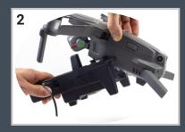
Slide the Automoving light unit above the belly of the aircraft above the rear aircraft arm while maintaining a 45° angle. As you do this, begin to adjust the Automoving light unit's angle so that, after the end of the sliding motion, it is parallel to the aircraft's body.
