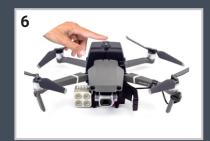
Hold the power button on the battery down for around 3 seconds to turn on the Automoving light. On startup the floodlight LED will blink once, when the boot sequence is ready the lamp will blink one more time.
