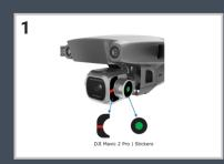
Mount the green tracking mark sticker aligned to the circle on the aircraft's camera. Mount the red tracking sticker on the aircraft's camera (see illustration).
