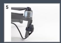
Slide the cable plug upwards until it reaches the front LED. Slide it upwards until it fully covers the aircraft's front LED. Fasten the cable below the drone's arm with the Velcro. Connect the USB C connector to the USB C port on the Automoving Light.
