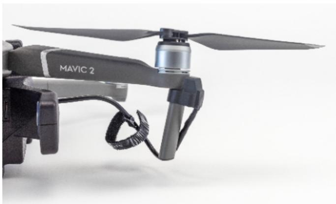
Loosen the Velcro that is attached to the cable
