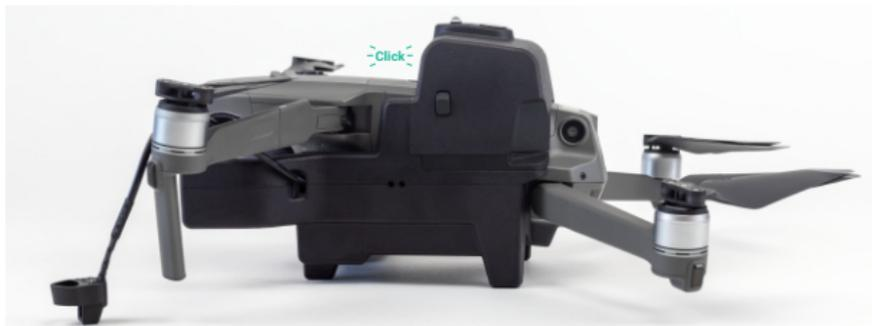
Make sure the battery is mounted securely and that the Battery Latches have "Click" into place on both sides.
