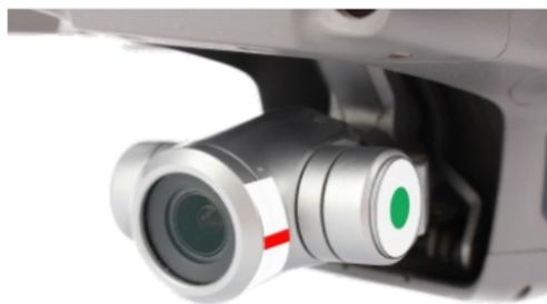
Tracking marks mounted on a DJI Mavic 2 Zoom's camera.
