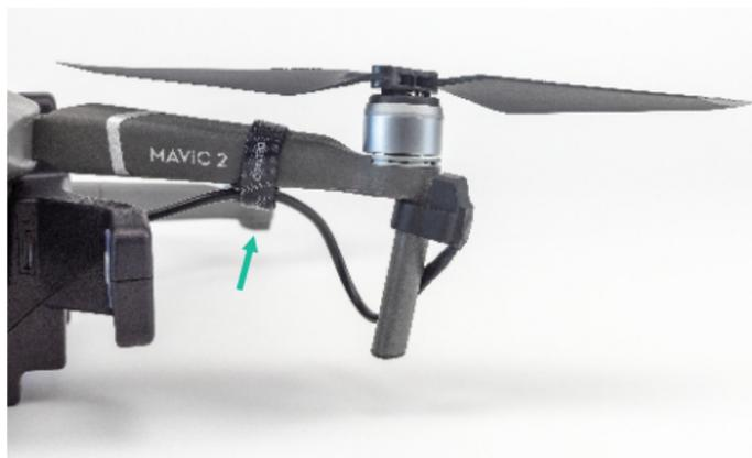
Fasten the cable below the drone's arm with the Velcro.
