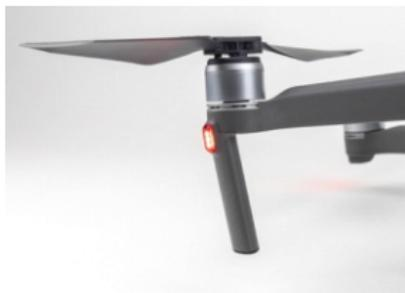
Turn on the aircraft's front LEDs with the Remote controller's C2 button.
