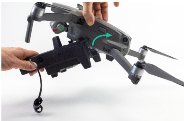
Hold the Automoving light unit in a 45-degree angle and slide it above the aircraft's body above the rear aircraft arm. While doing this, simultaneously start to change the angle of the Automoving light unit so that it is positioned in parallel with the aircraft's body at the end of the sliding movement.
