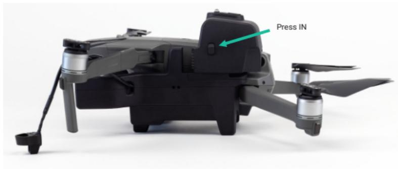
Press IN the "Battery Latches" on both sides of the battery and position the Battery with the Automoving light unit battery slots
