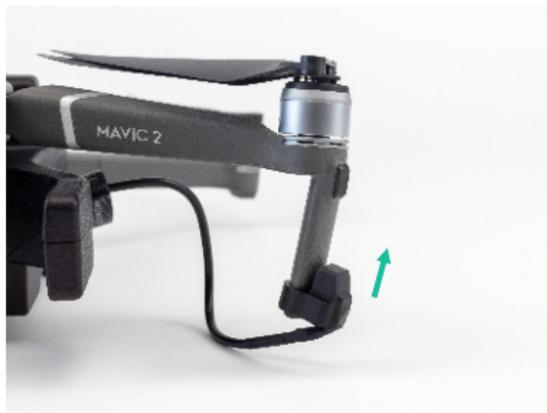
Lift the aircraft's front leg and place the cable plug at the bottom with the cap facing upwards.
