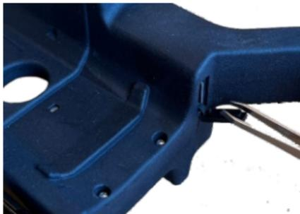
Use tweezers or other suitable tool to pull out the SD card without damaging it
