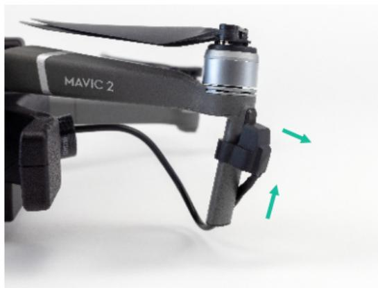
Slightly lift the edge of the cap to be able to slide the cable plug fully above the front LED.
