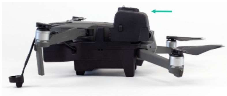
Slide the battery forward along the battery slots into the Automoving light unit until it locks.
