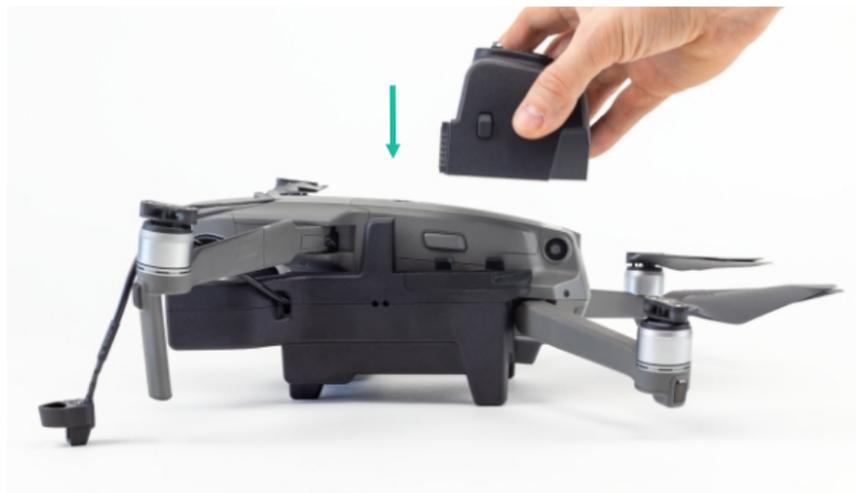
Insert the Automoving light Battery into the Automoving light's battery slots.
