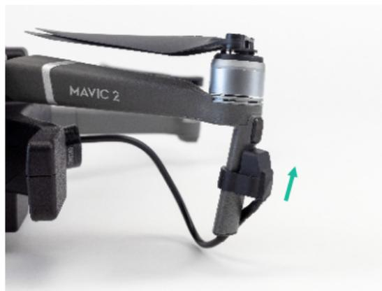
Slide the cable plug upwards until it reaches the front LED.
