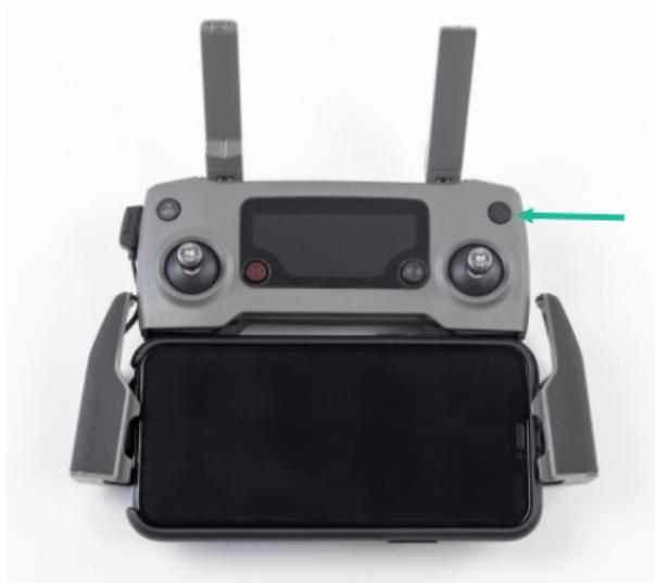
Turn on the aircraft's Remote controller and make sure it connects to the aircraft.
