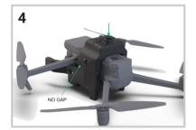
When correctly mounted, there should be no «GAP» between the battery and the battery connector on the Automoving light unit. Hold the power button on the battery down for around 3 seconds to turn on the Automoving light. On startup the floodlight LED will blink once, when the boot sequence is ready the lamp will blink one more time.
