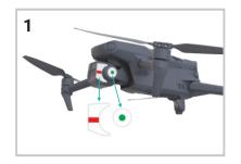
Mount the green tracking mark sticker aligned to the circle on the aircraft's camera. Mount the red tracking sticker on the aircraft's camera (see illustration).
