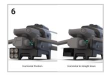
Power up the aircraft and make sure that the DJI Fly app connects to the aircraft. Tilt the «Drone Camera» by pressing the «C2 button» horizontal to straight down and back within 2 seconds with the DJI Remote controller (the flood light will turn «ON/OFF» after Automoving light is mounted to the drone successfully).
