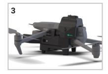
Place the Automoving light Battery into the Automoving light's battery slots' starting point. Press in the «Battery Latches» on both sides of the battery and slide the battery. Make sure the battery is mounted securely and that the «Battery Latches» have clicked into place on both sides.
