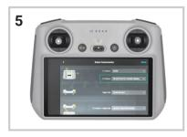
Set the function of the customizable «C2 button» in the DJI Controller to turn on/off the «Recenter/Tilt down gimbal». The light is toggled when the camera goes from horizontal to straight down and back to horizontal within 2 seconds, this is done by clicking the C2 button two times within 2 seconds.
