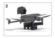
Position the Automoving light unit below the aircraft. Insert the aircraft from above into the Automoving light's inner body.
