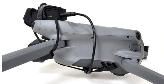
Once the top hooks are hooked to the position, pull the bottom hooks and hook them to the third ventilation pocket on both the left and right side of the Drone, as shown in the image
