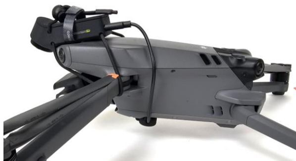
Once the top hooks are hooked to the position, pull and push the bottom hooks down by aligning the two fins of the Activator to the slots in the Drone.
