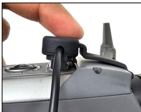
Once the top hooks are hooked to the position, pull and push the bottom hooks down by aligning the two fins of the Activator to the slots in the Drone.
