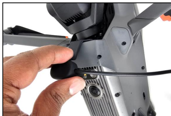
Using the hand, hook the activator to the top side of the Drone as shown in the image
